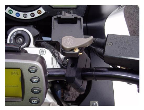
On the right picture you can see the rubber plate between the tilthead and the barholder. To see the shim you need some phantasy.
